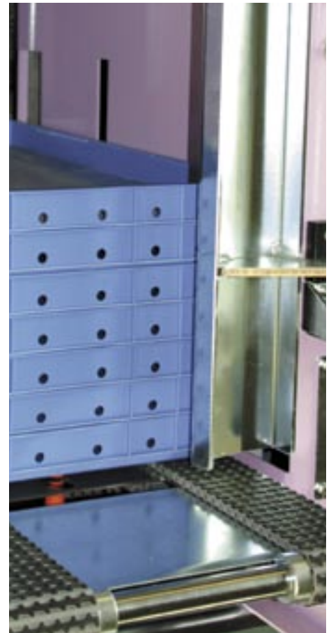
A 152 mm (6.0 in.) uni M-QNB Rubber Top is used to pull light-weight boxes from a stacker
